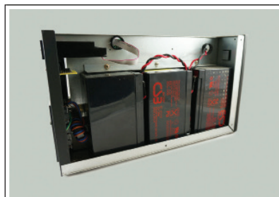
Replacement batteries for the UPS
